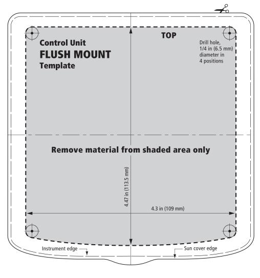
FLUSH MOUNT template for ST60+ Instruments
