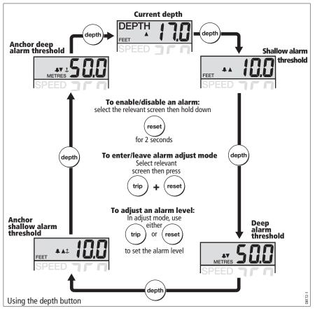
You can enable and disable individual alarms by pressing the **reset** button for 2 seconds, while the relevant alarm screen is displayed.
