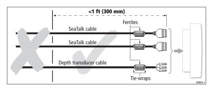
**Note:** It is NOT necessary to fit a ferrite to the Speed transducer cable.
