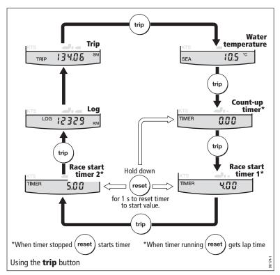
To reset a timer to the start value, stop it then hold down the **reset** button for 1 second.
