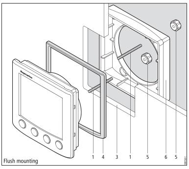
8. Locate the flush mount bracket (6) onto the fixing studs and secure the assembly to the panel with the thumb-nuts (5).
